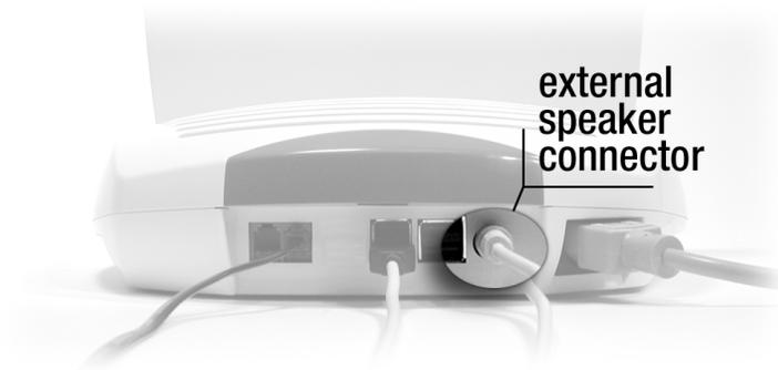
1. Plug the speaker cable into the speaker connector shown in the graphic above. Make sure that your port connector is seated properly.
