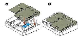
Use shorter **flat head screws** to fasten Raspberry Pi and HDMI Board assembly to top case.
