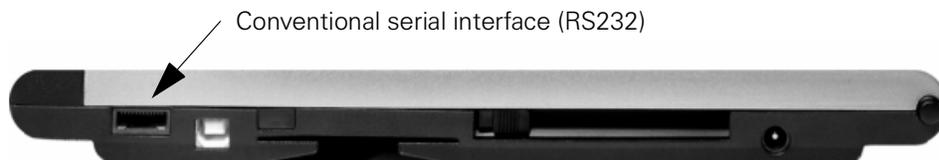
**Serial Interfaces for connections to the PC**
