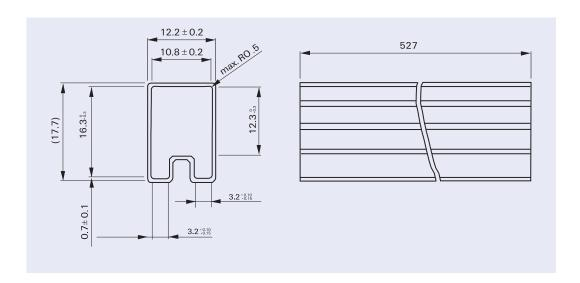
Tube for THT version 25 relays per tube 1'000 relays per box
