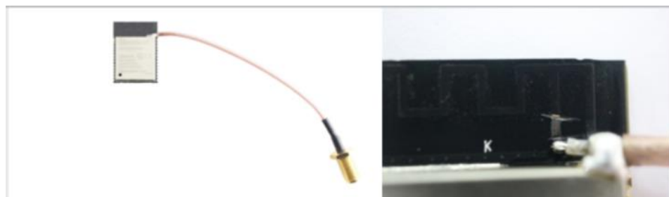
Figure 2-2. RF Cable Connection for Module Conduction Test
