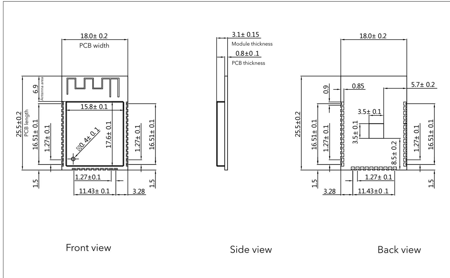
Figure 6: Dimensions of ESP32-WROOM-32D
