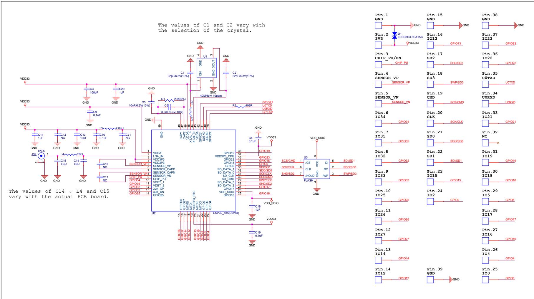
Figure 4: ESP32-WROOM-32U Schematics
