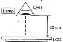
The distance between LCD panel and Lamp and also human eyes is around 30 cm.
