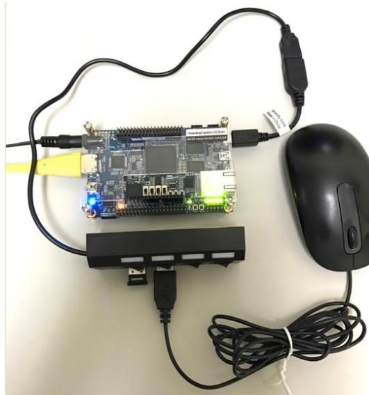
**Figure 2 DE10-Nano Demo Setup**
