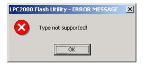
After "OK" is pressed in the above message, the ISP commands will still be executed and the Part ID and the Boot loader ID will be displayed.
