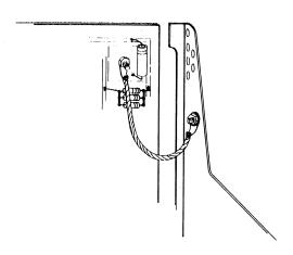
NOTE: At any point where a connection is made to the chassis, first rub the area around the connection point with sandpaper or some other abrasive to remove the anodizing.
