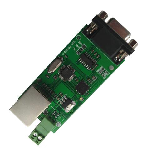
Notice: USR-TCP232-2 is a base version of USR-TCP232-24, the difference from USR-TCP232-24 is no RS485 interface, their usage is the same, so please reference to USR-TCP232-24 data sheet.
