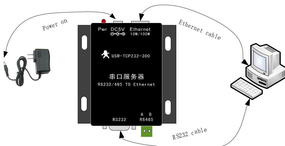
3. Setup the PC IP address to 192.168.0.201
