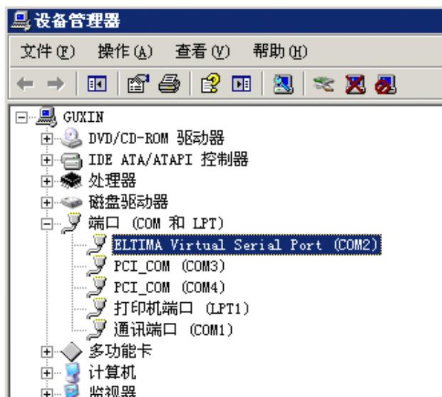
At this point, you can use your equipment as an ordinary serial port, and operate of local virtual serial port will converted to operation of the remote module RS232. The figure is show send data between the two serial port.
