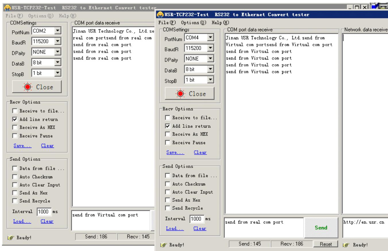
Test 100ms recycle send, send and receive 10,000 bytes, every thing is ok.
