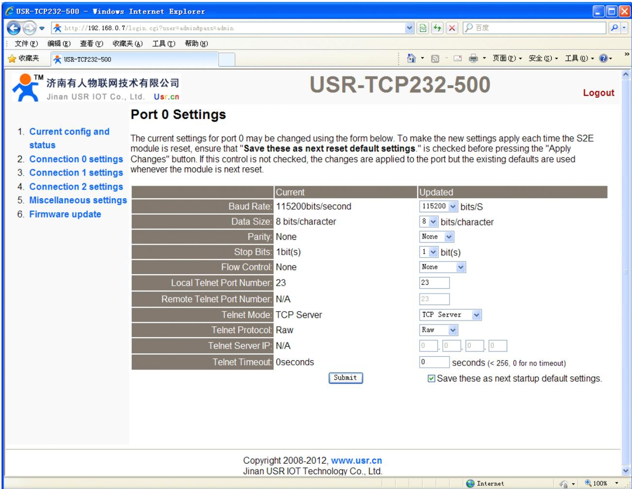
The default working mode simply test, on the basis of hardware connection, then connect USR-TCP232-500 COM1 with the computer, use the software USR-TCP232-Test in CD to test. The left is serial port, using software default settings, the right is network, set to be TCP Client, the server is IP 192.168.0.101 that you got just now, port number 23.
