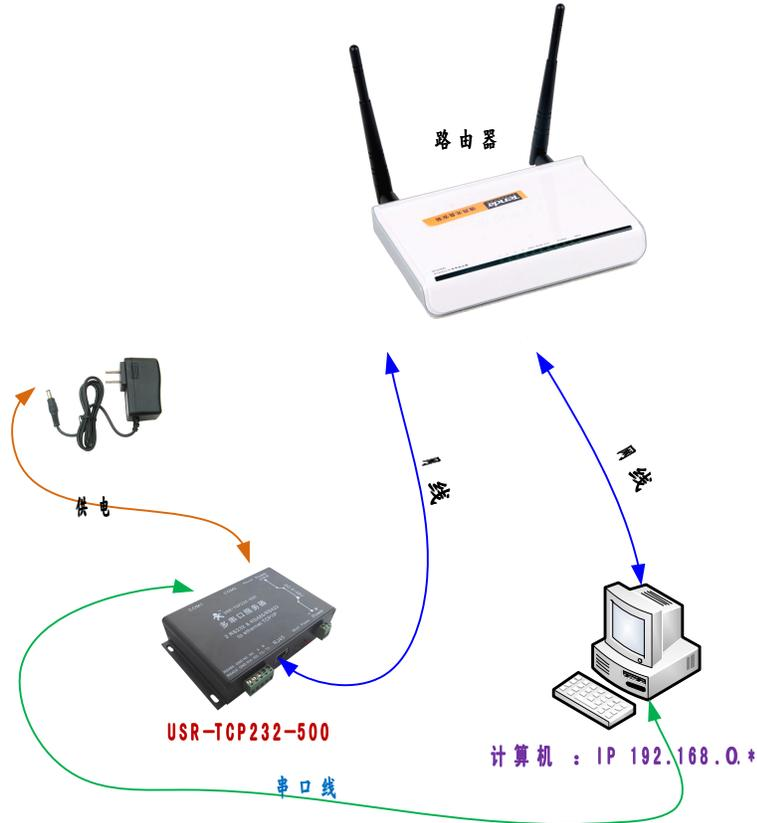
Through the router ( picture above) or directly connected with computer ( picture below)
