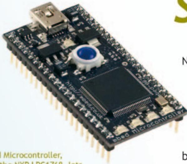
The mbed Microcontroller, based on the NXP LPC1768, lets you work with an ARM Cortex-M3 in a 0.1" DIP form-factor. Combined with the <http://mbed.org> website, featuring the mbed "Cloud" Compiler, it is an ideal platform for rapid prototyping with microcontrollers.
