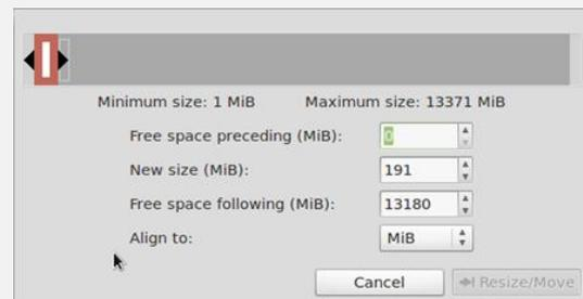
In the Free space following (MiB) type 0 and press enter, or grab hold of the partition (at the top) with your left mouse button, and drag it all the way to the right:
