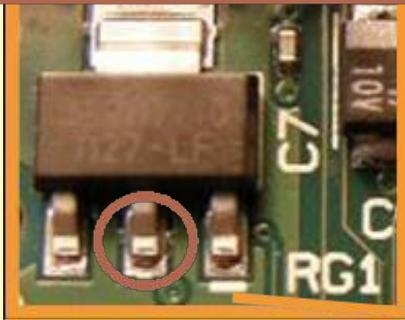
**2V5 Pin 5 of RG3** (LP2980 Voltage Regulator) used for Composite Video Out
