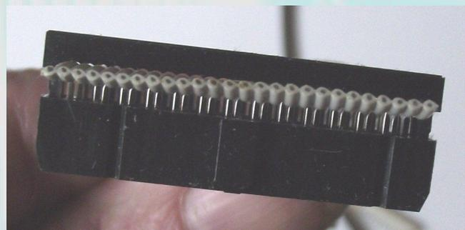
7. Insert the 26 way ribbon into an IDC connector, ensuring the marked wire and the marked pin (wire 1 and pin 1) are lined up. Leave a little bit of cable protruding through the connector.
