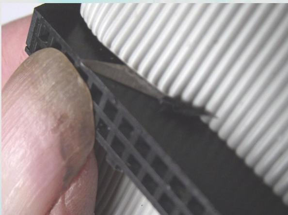
4. Now carefully trim the cable ends as close to the connector as you can with the modelling knife.
