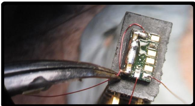
When under a 10X scope I have used worn tips (like old nails) because the magnification allows you to position a bad tip well. Despite this I have a file which I use to shape my tip to a fine point. This is done when the iron is cold/off.
