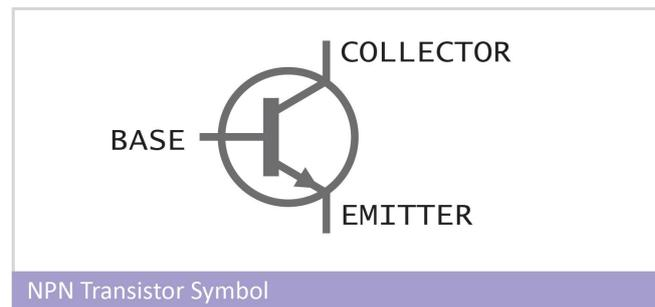
Base & Emitter. When a small current is applied to the Base terminal it allows a much larger current to pass between the collector and emitter terminals.
