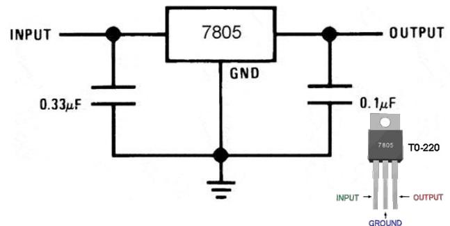
With an input voltage higher than 7V, you will have a 5V regulated output voltage for the Pi.
