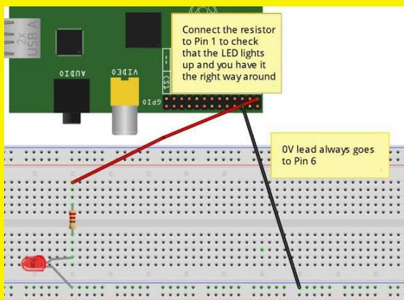
**Figure 1 - LED Test**
