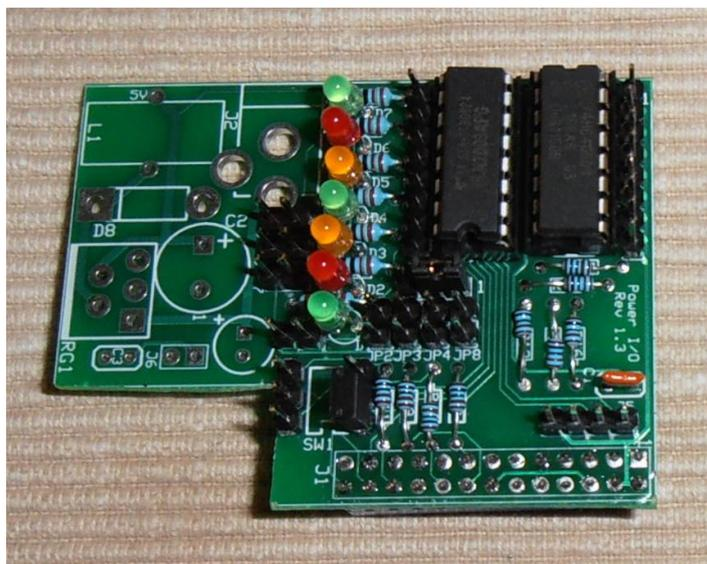
A hexadecimally encoded switch (SW1) can be included if the intended application appreciates its functional or educational value but it has been omitted from the unit pictured above for budgetary or functional reasons, replaced by a pair of 3-pin headers that can be jumpered to match user requirements.
