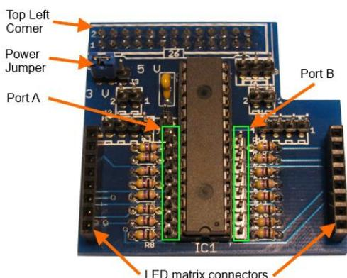
Push the two female header strips onto the LED matrix, then solder them to the PCB. This ensures perfect alignment. Remove the LED matrix. Finally, solder the 26-pin female header. **NOTE:** Unlike all the other components, this header is placed on the underside of the PCB and soldered on the top side.
