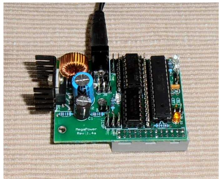
The MegaPower unit pictured above is complete and being tested in standalone operation. The heat sink (far left) is needed if MegaPower is providing power for a Raspberry Pi Model B but should not normally be required by a Raspberry Pi Model A or for standalone operation. Near the right edge of the PCB there is provision for 2 pull-up resistors (R6 & R7) that may be required by
