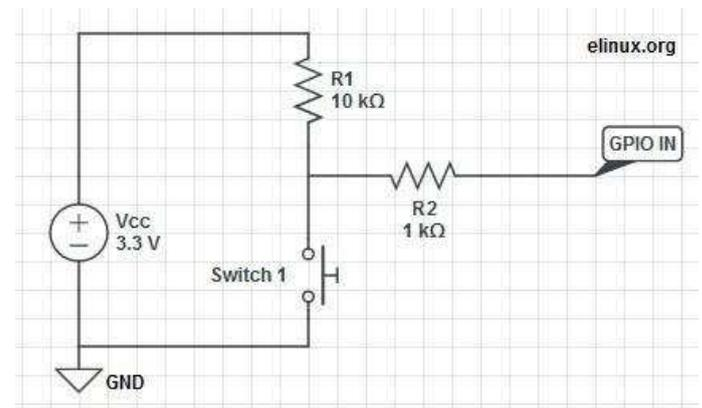
When a GPIO pin is set to input, it doesn't provide any power and consequently has no distinct voltage level; defined as 'floating'. We need the pin to be capable of judging the difference between a high and low voltage, however in a floating state it's liable to incorrectly detect states due to electrical noise. To enable the pin to see the difference between a high or low signal we must 'tie' that pin, calibrating it to a defined value; 3.3V in this case!
