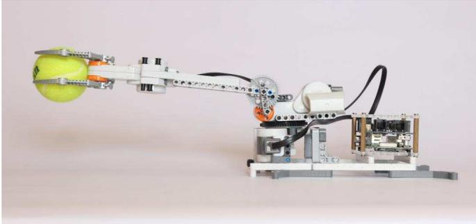
This example uses the BrickPi as a robotic arm for grabbing and moving materials. In this example, a keyboard connected to the Raspberry Pi is used to control the movement of the arm.
