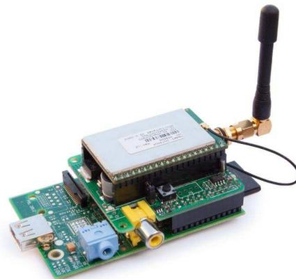
One feature I wanted was for the remote radio to be able to control power to the remote Raspberry Pi. This would be very useful for turning the Raspberry Pi off when not needed, saving battery power. Later, I also added a real-time clock, a useful feature which allows the Raspberry Pi to keep time without a network
