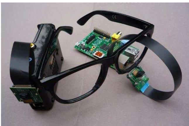
For more serious research, frame rates faster than 30 are desirable, and it is hoped that for formats considerably smaller than 1080HD, 60-90fps may be available shortly. The sensor is capable of 500fps for some formats, and this would allow one to estimate accelerations as well as velocities and locations.
