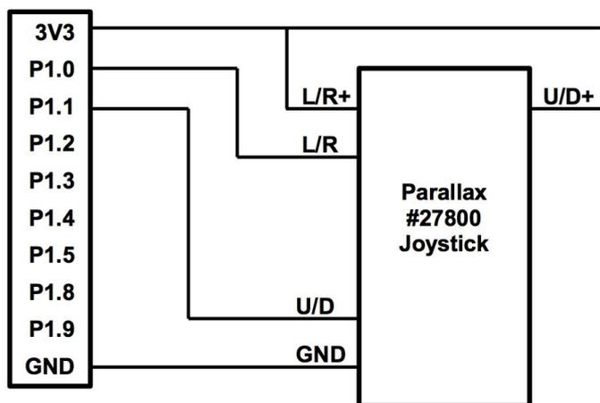
Figure 2 MJoystick Connections
