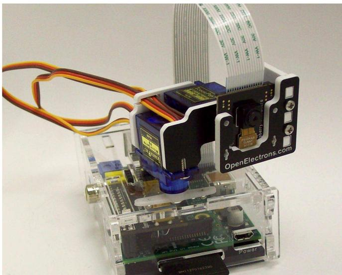
There is a programming interface for these servos and the position of each servo can be controlled through a Python program. This gives you the ability to point your camera in a precise direction.
