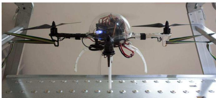
The code changes in "TESTCASE 3:" disable the front-right and back-left motors. Place these arms on the two platforms such that your quadcopter dangles in free space between the platforms as shown in the photo. The other two motors will spin at your newly found `cli_hover_speed`. Your quad may not balance between the platforms unless gently supported by you. Enter:
