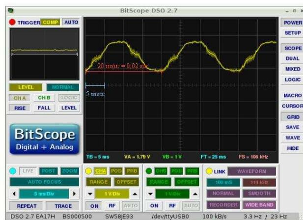
**Figure 5:** Determining the frequency of a signal
