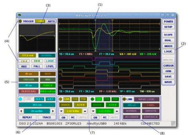
**Figure 2:** BitScope DSO software main screen elements (photo courtesy by BitScope Designs)
