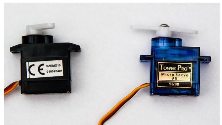
Figure 4 - Small servo motors
