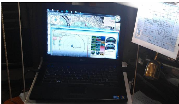
The laptop can use TCP to receive data from the Raspberry Pi and present it simultaneously in my Graphical Console, and the popular open source package OpenCPN (Open Chart Plotter Navigator).
