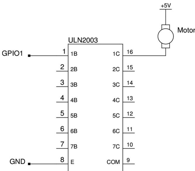
Figure 2 - ULN2003 and small DC motor
