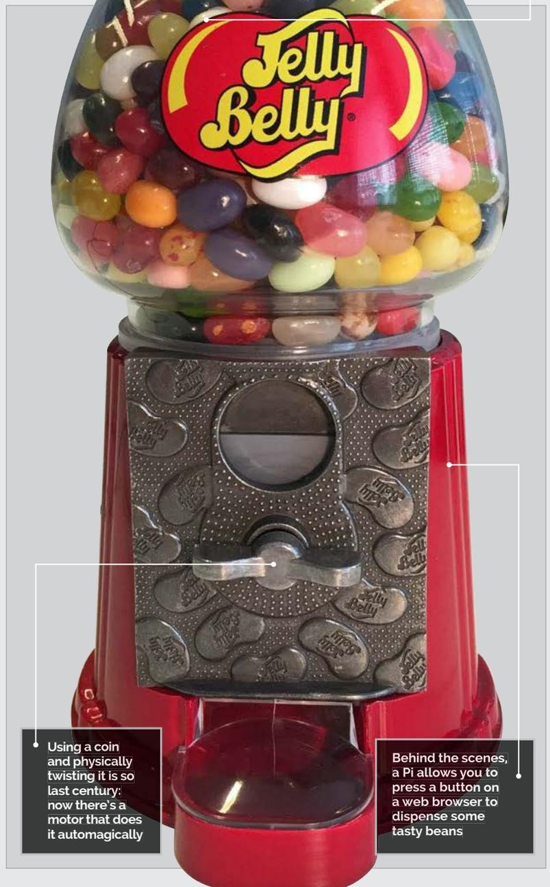
Using a coin and physically twisting it is so last century; now there's a motor that does it automatically
