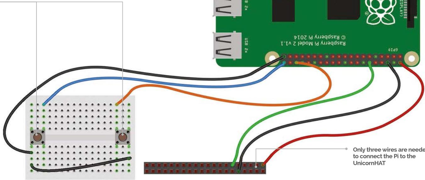
Only three wires are needed to connect the Pi to the UnicornHAT
