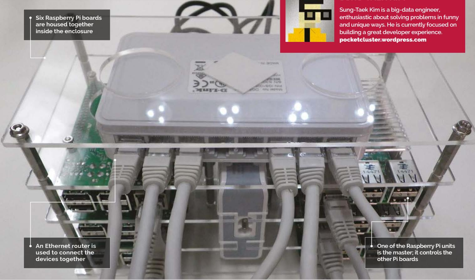
• Six Raspberry Pi boards are housed together inside the enclosure
