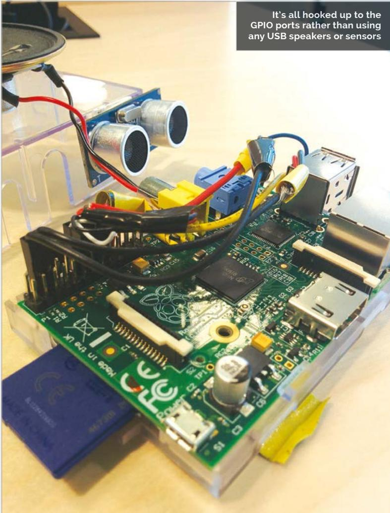
It's all hooked up to the GPIO ports rather than using any USB speakers or sensors
