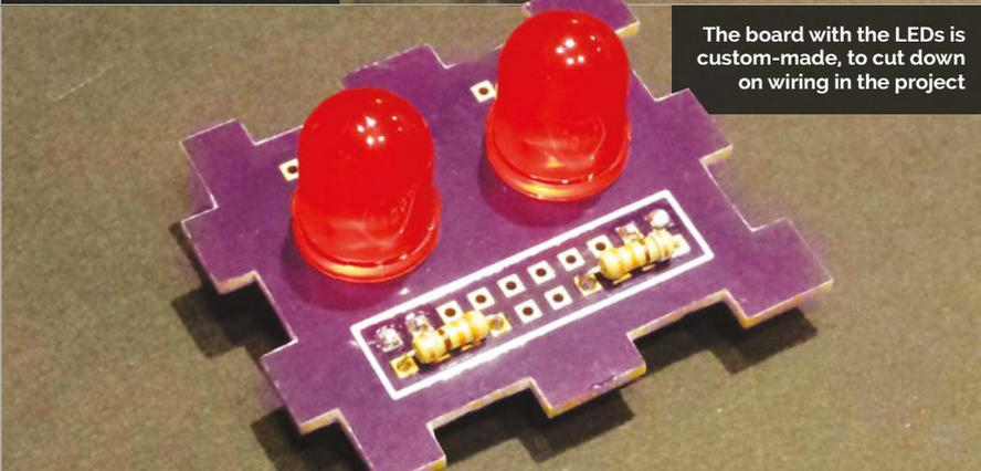
The board with the LEDs is custom-made, to cut down on wiring in the project
