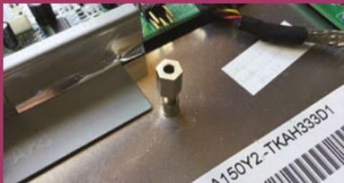
With the back off the VGA monitor, it revealed two short tapped pillars. We extended these with a 10mm M3 tapped pillar, fastened with a piece of M3 studding or thread cut from a longer bolt. This was the basic anchor for the system. It was fastened to a length of 30x12 aluminium channel of 3mm thickness that spanned the whole width of the frame. The channel walls were trimmed to fit flat.
