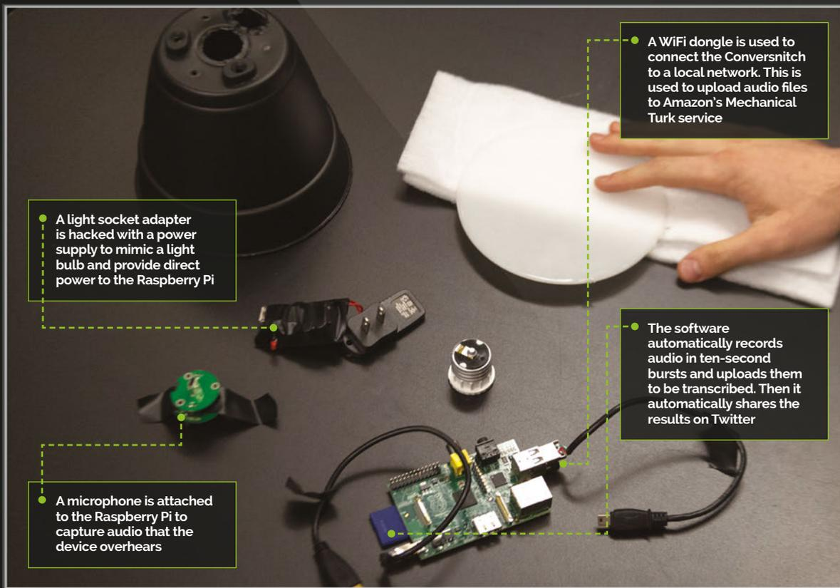
● A light socket adapter is hacked with a power supply to mimic a light bulb and provide direct power to the Raspberry Pi
