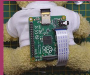
to get it to launch at boot. It's also a good idea to go to Raspberry Pi Configuration and have it boot to the CLI; this means it will turn on a bit faster and use less power, as you won't need to use the graphical interface with this Pi. You'll still be able to dial in via SSH, though, for any maintenance.
