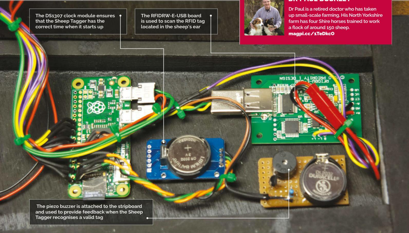
The DS1307 clock module ensures that the Sheep Tagger has the correct time when it starts up
