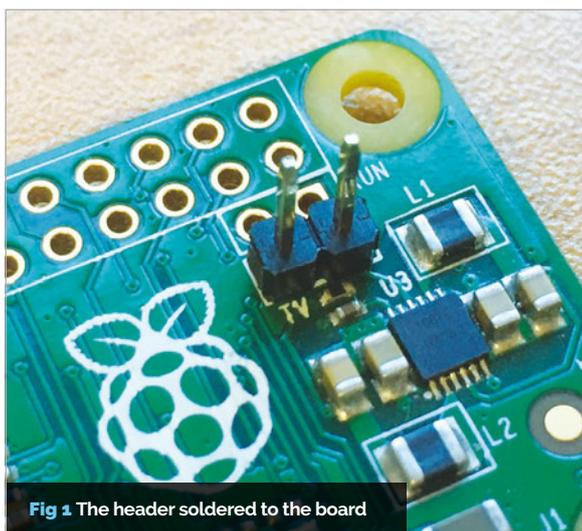
Fig 1 The header soldered to the board
