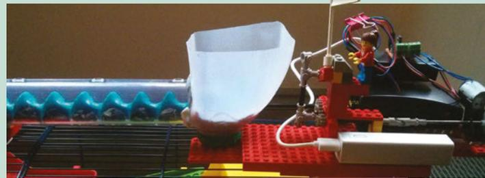
As our motor still runs too fast, we used technical Lego gearing to reduce the speed.
