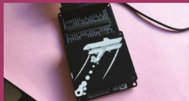
The Skywriter HAT was mounted on a Black HAT Hack3r extension board and fastened to the underside of the frame. You could just use a 40-way female-to-male ribbon cable if you want, but make sure the HAT is connected to the correct pins if you're doing this. Fit the frame glass with mirror film. Unfortunately, the Skywriter doesn't work from behind this film, which is why it's on the side.
