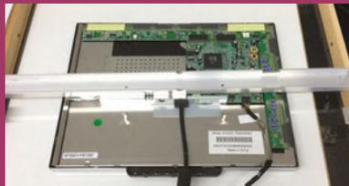
At each end, a piece of 20mm angled aluminium was mounted so that it could be bolted onto the frame with two M3 bolts. Holes in the top were used to fasten this to the long channel to make a secure fit. We found it a bit fiddly to hold the nuts on the underside of these right-angled brackets, so we fastened them on the underside with hot-melt glue to allow easy assembly and disassembly.
