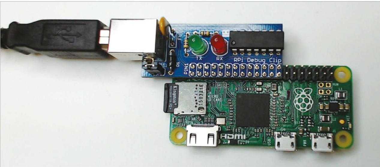
**Left** Make sure that JP1 in the Debug Clip is closed, as this will allow you to power the Pi Zero directly from the Debug Clip
