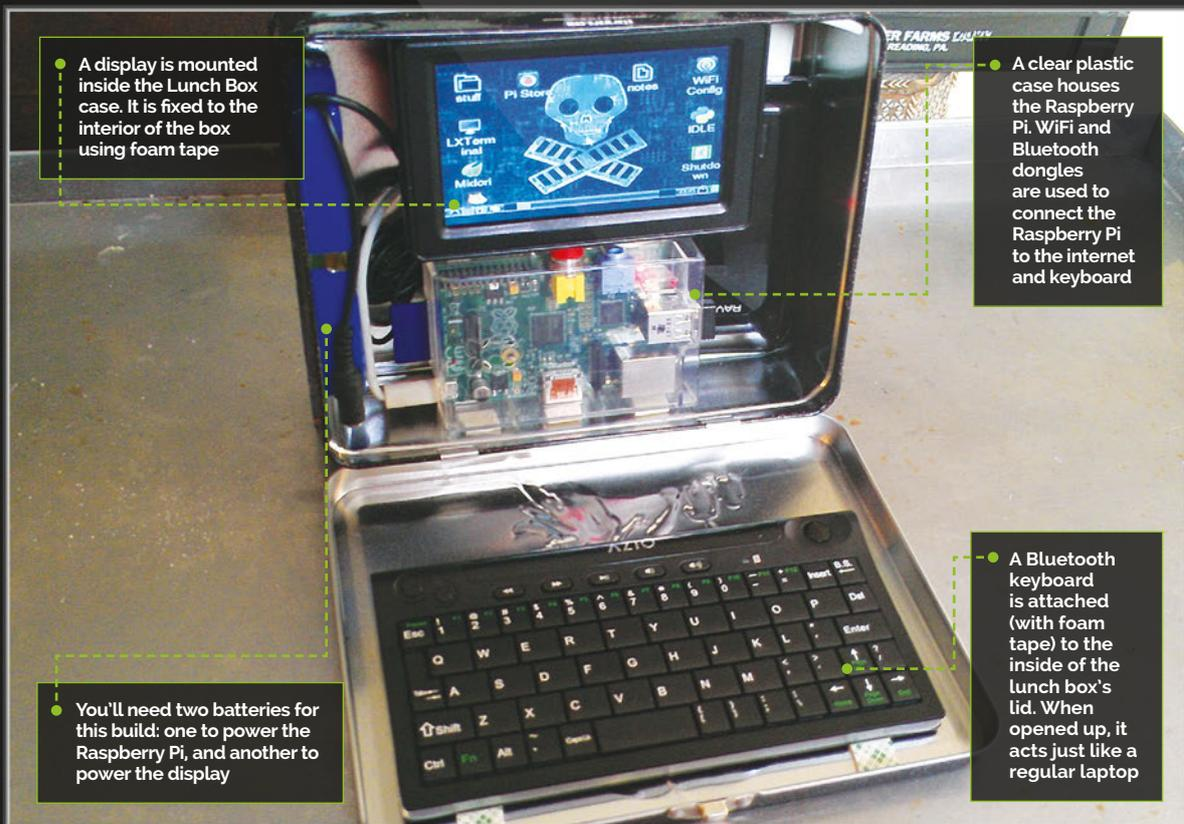
A display is mounted inside the Lunch Box case. It is fixed to the interior of the box using foam tape
