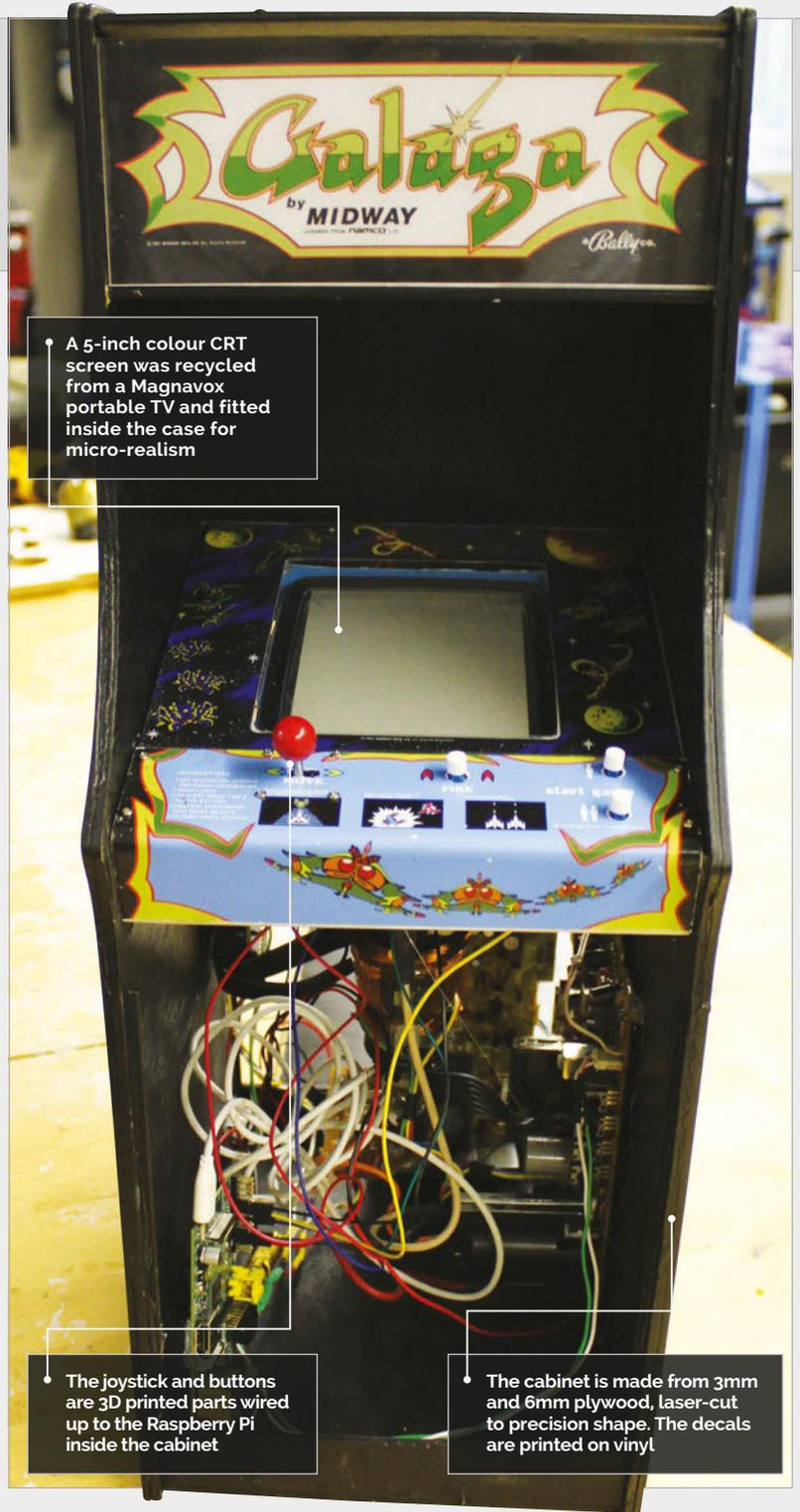
• A 5-inch colour CRT screen was recycled from a Magnavox portable TV and fitted inside the case for micro-realism
