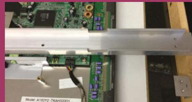
Slots were cut in the wall of the channel to allow cables to pass through, and also allow clearance for some components on a side board. Don't cut too deep or you'll start weakening the beam somewhat – in the long run, that would be bad for the overall structural strength of the mirror, and that wouldn't make your life easier in the way we want.
