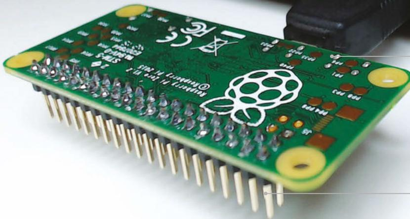
Use the micro USB data port for both power and Ethernet connection
