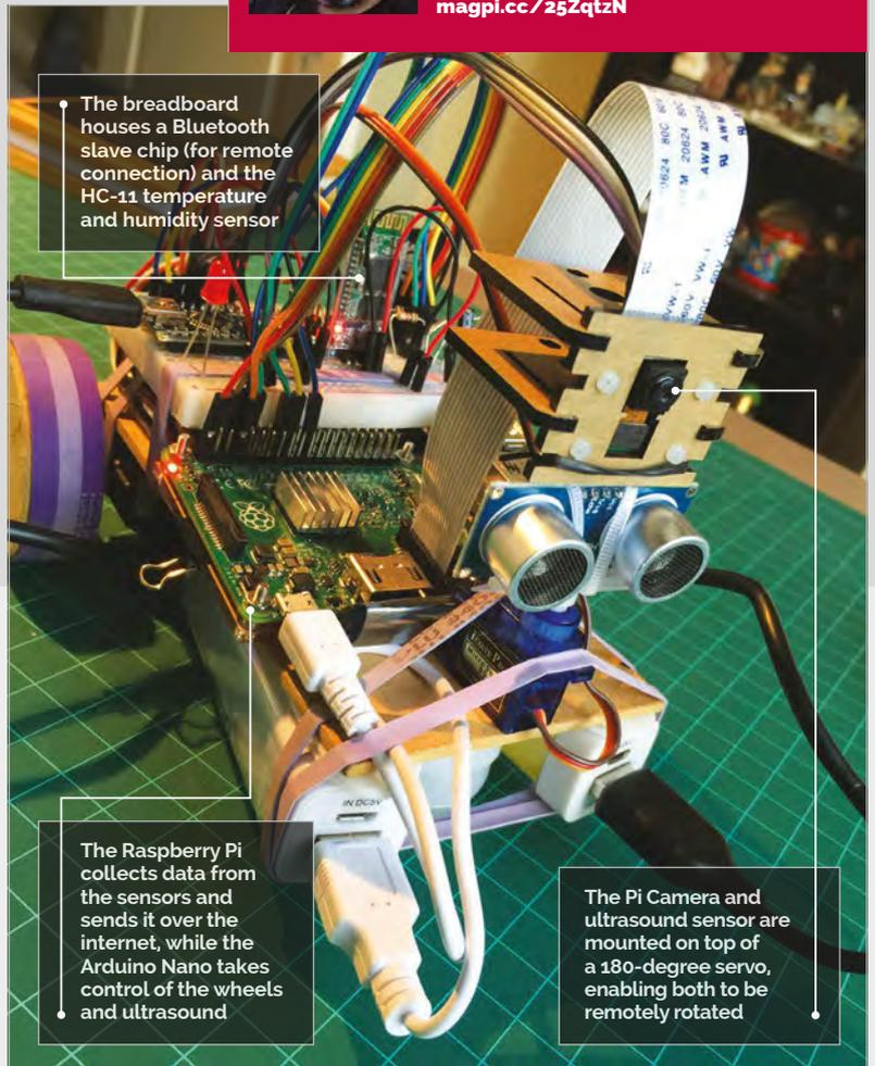
The breadboard houses a Bluetooth slave chip (for remote connection) and the HC-11 temperature and humidity sensor
