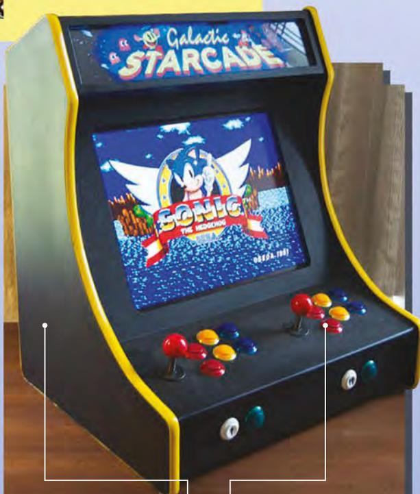
The cabinet is made from regular MDF (medium-density fibreboard) cut to shape and glued together
