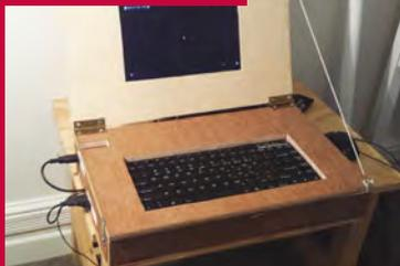
According to user gepset on Reddit, his school instituted a bring-your-own-device (BYOD) policy. Being a poor student, he made this wooden Raspberry Pi laptop from scratch. It folds, has access to all the necessary ports, and features a keyboard. A great little device!
