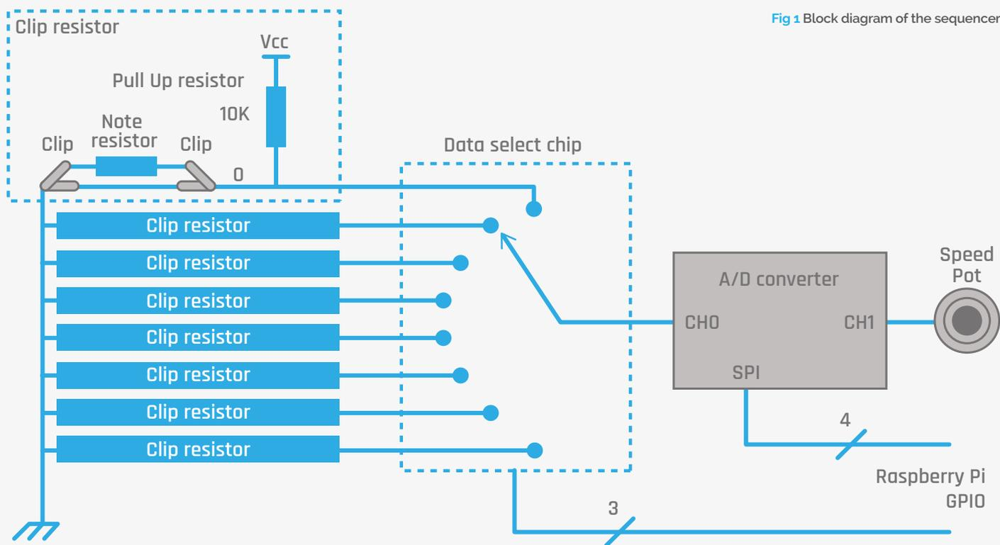
Fig 1 Block diagram of the sequencer
