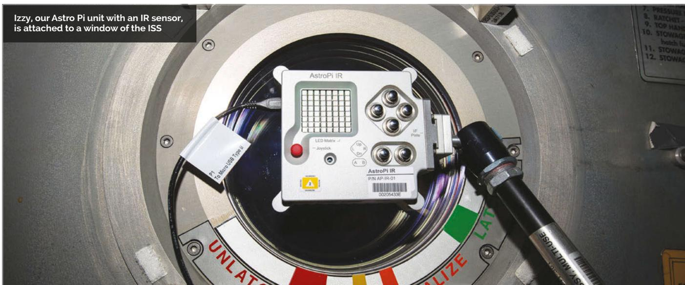
Izzy, our Astro Pi unit with an IR sensor, is attached to a window of the ISS
