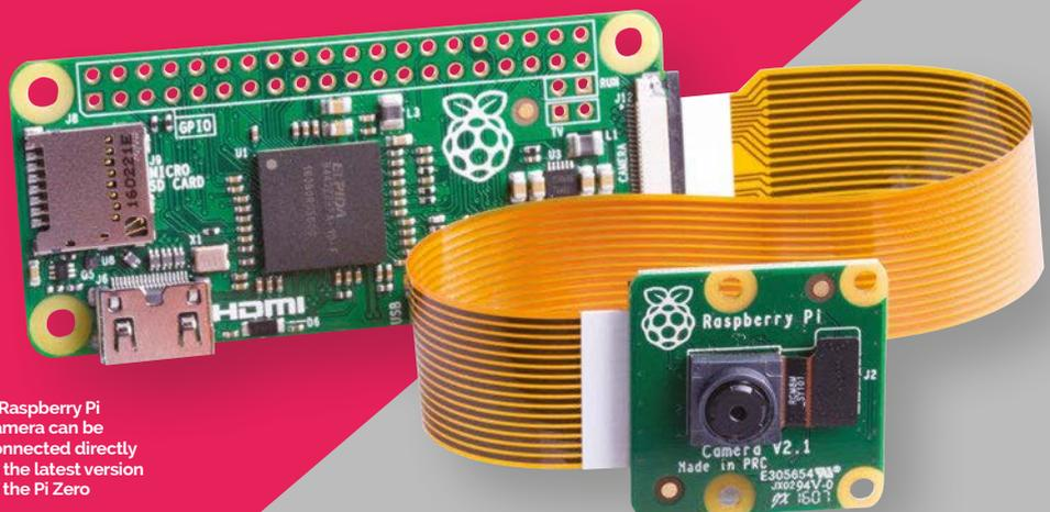
A Raspberry Pi camera can be connected directly to the latest version of the Pi Zero
