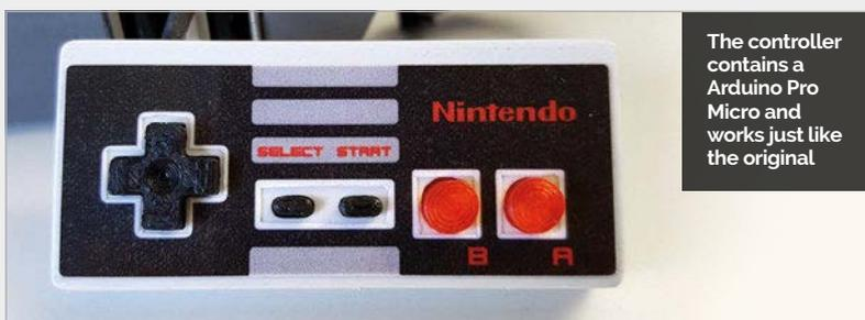
The controller contains a Arduino Pro Micro and works just like the original
