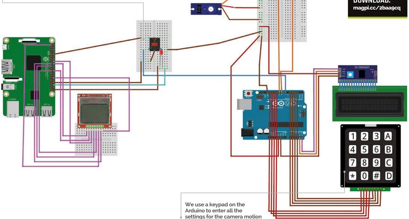
We use a keypad on the Arduino to enter all the settings for the camera motion
