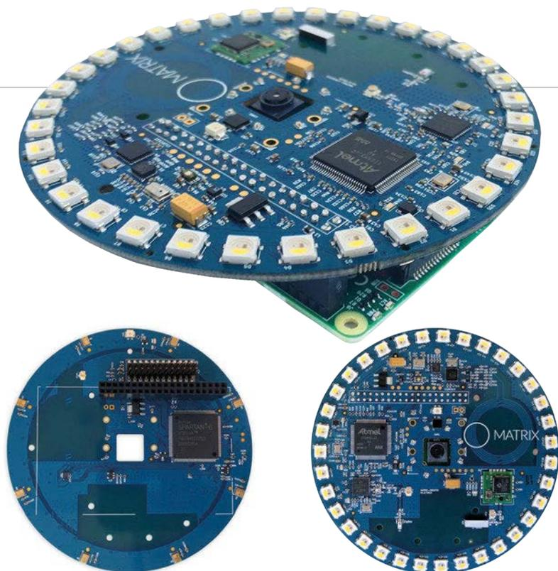
**Above** The MATRIX has many functions, including a multitude of sensors and microphones, as well as a ring of LEDs around the edge
