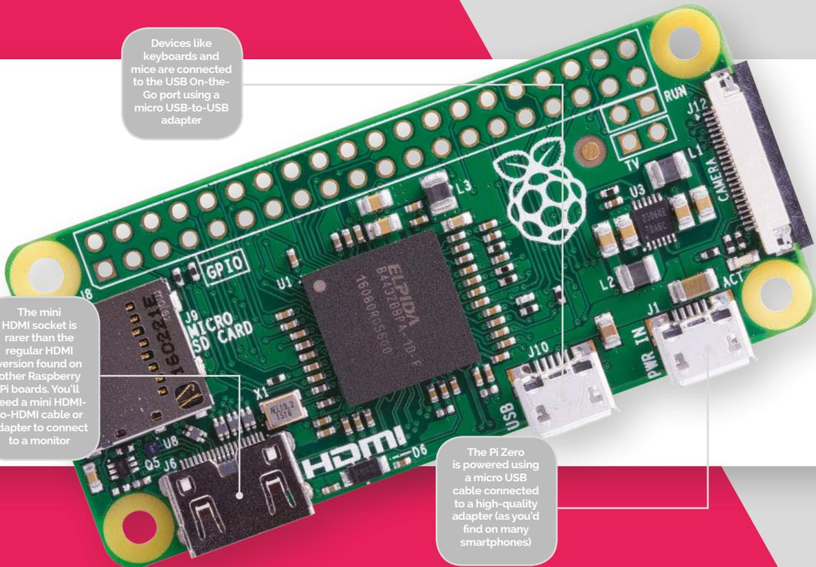
The Pi Zero board uses the same micro USB power input as other Raspberry Pi devices, and you can
