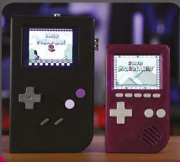
It's been through a few iterations, and the latest Pocket PiGRRRL uses a Raspberry Pi and PiTFT HAT (320x240 pixels) to create a portable gaming console.
