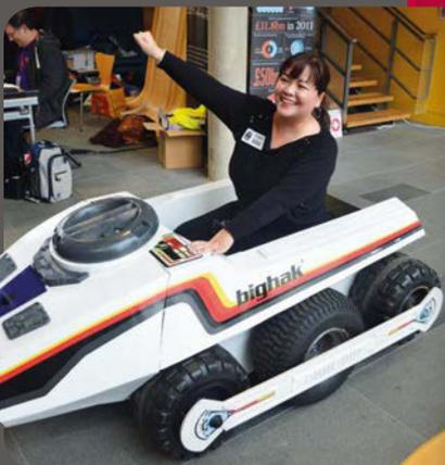
commands by holding up QR codes to the webcam. A Raspberry Pi turns the commands into directions and Bighak trundles off.
