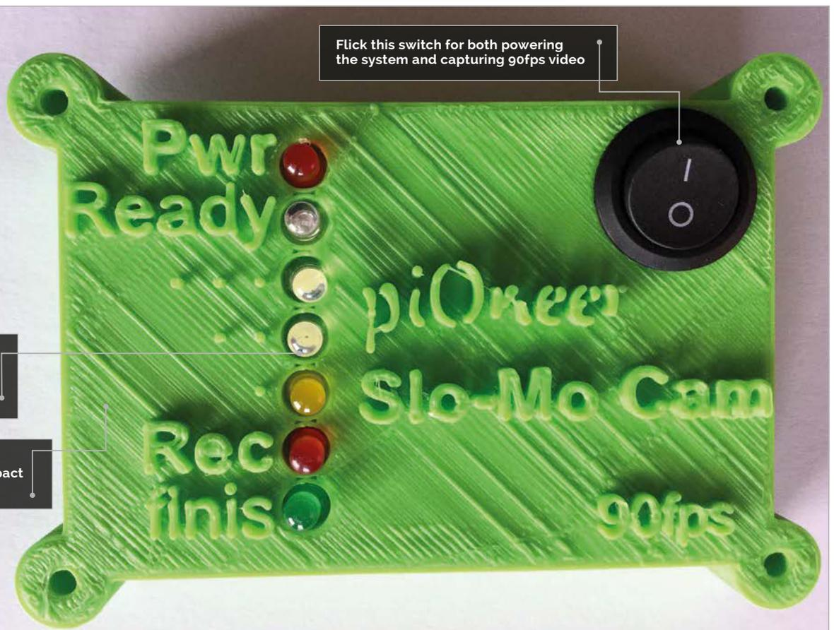
This row of LEDs is the user interface for displaying the camera's status
