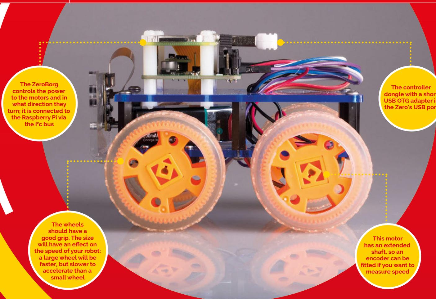
The ZeroBorg controls the power to the motors and in what direction they turn; it is connected to the Raspberry Pi via the I<sup>2</sup>C bus
