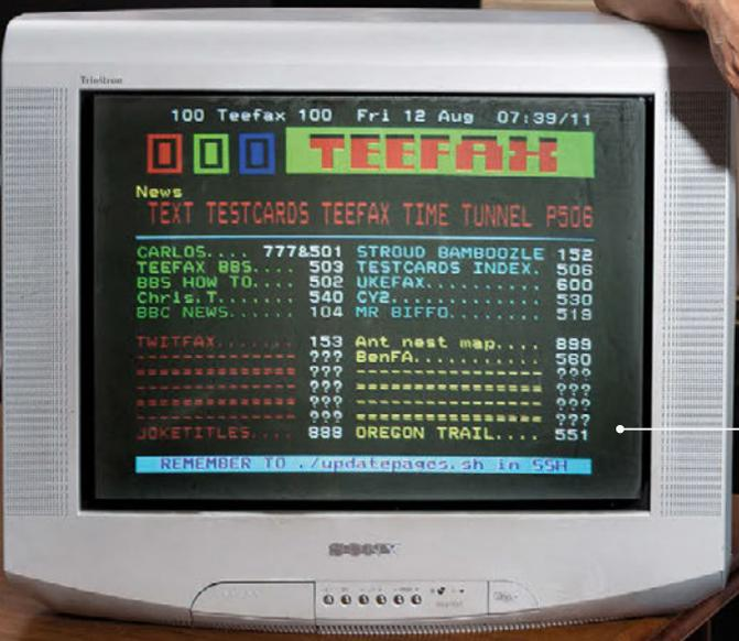
The data transmitted via the Pi's composite video signal is converted into teletext pages
