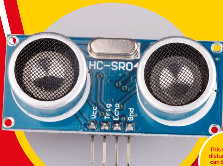
This ultrasonic distance sensor can be used to check how far away the wall is
