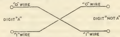
FIG. 10/4. Logical element Not or Complement of
