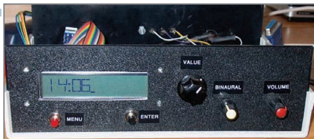
Photo 1—This is the relaxation generator's front panel.
