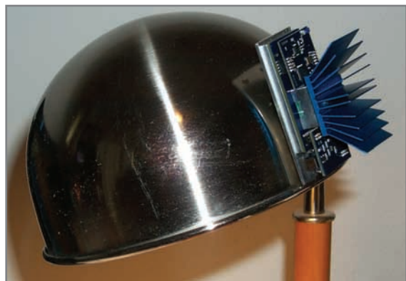
Photo 4 —Despite an extremely poor fit (i.e., thermal interface) between the NODE baseplate and curved hood of the desk lamp, this setup easily generated enough power to run the demo.
