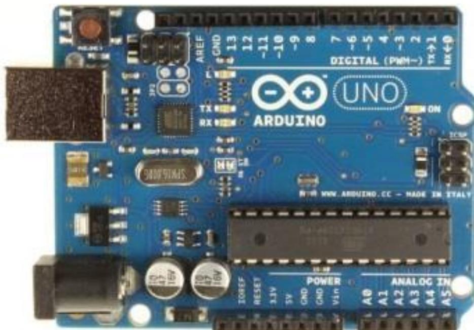
Arduino UNO R3 board with ATmega328P – ([Click to see on Amazon](http://amzn.to/YMjZq) <http://amzn.to/YMjZq>)
