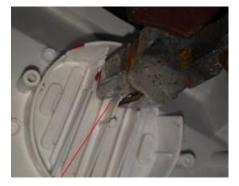
Use the wire snippers to cut away the plastic loudspeaker mounting on the bottom of the Big Trak.
