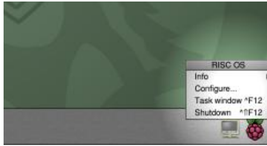
Select 'Task window' from the Raspberry menu to access BBC BASIC in RISC OS.
