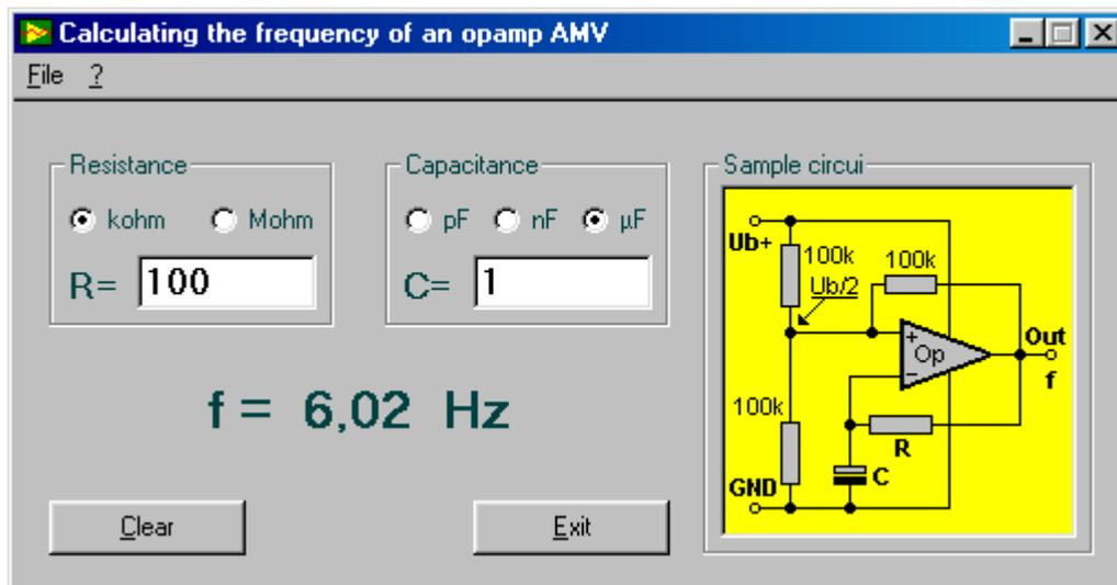
The opamp is wired as shown in the circuit diagram. This means that half of the supply voltage ( $U_b$ ) should be connected to the non-inverting (+) input, with a negative-feedback resistor connected to the output. Normally, a value of  $100\text{ k}\Omega$  is used for all three of these resistors.
