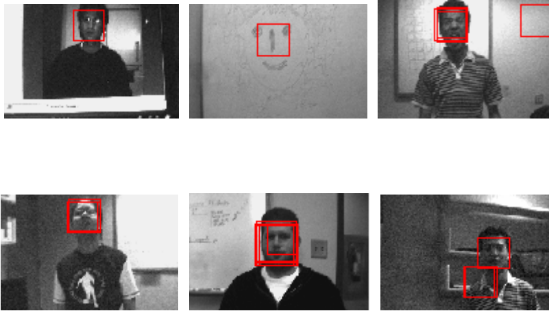
Fig 6. Detected Faces from CMUcams3 Face Detector
