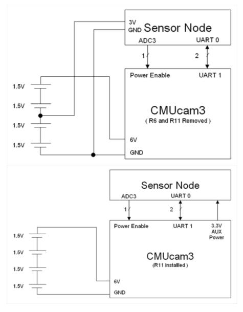
This images shows how to connect a Tmote Sky board to the CMUcam3. Note, that the battery has been removed and a receptical (S6105-ND from <a href="Digikey">Digikey</a>) has been soldered onto the bottom side of the Tmote Sky board.
