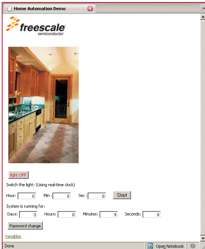
Figure 7. The first web page the user sees when accessing DigiButler from a PC web browser. You can switch the kitchen lighting on and off.
