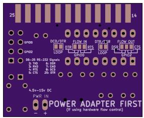
The underside of the modem contains several solder jumpers that enable you to customize the hardware flow control wiring to suit your application. The most typical settings are to use RTS/CTS hardware flow control.
