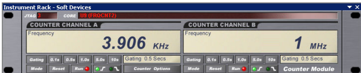
Figure 57. Frequency counter control panel
