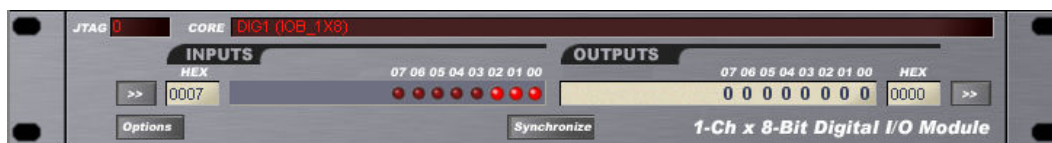
Figure 47. Digital IO module, used to monitor and control nodes in the design
