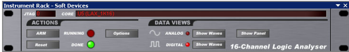
Figure 59. Logic analyser instrument control panel
