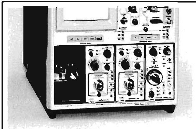
A. Installed Sampling Units.
