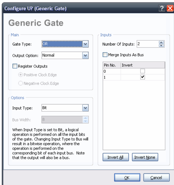
Figure 8. Configuring the GATE component as a 2-input OR gate with one input inverted.
