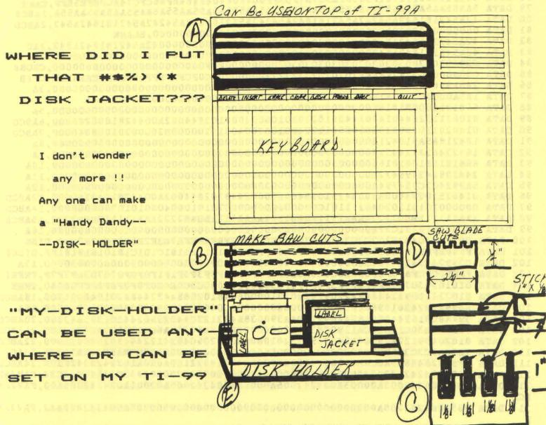
I USED A 2%1/4 INCH X 10 INCN-BLOCK OF WOOD SECAUSE IT WILL FIT THE TOP OF THE TI-99 CONSOLE. I DON'T BELIEVE IT WILL CAUSE ANY HEAT PROBLEMS IF YOU DON'T COVER THE AIR-VENTS AT THE TOP RIGHT SIDE.
