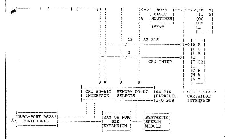
(THE SYSTEM BLOCK DIAGRAM CAN BE USED FOR REFERENCE WITH THE FOLLOWING SPECS)
