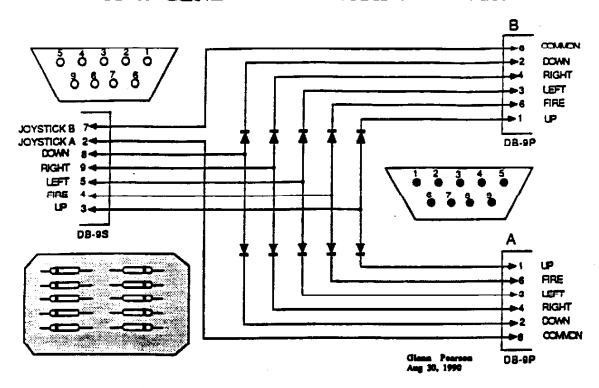
As virtually all T2 users know, standard joysticks may not be used with the TI (or Geneve) without an adapter. The adapter is required to accompdate three things; the pineut of the DB-9 connector on the TI does not match the standard joystick pineut, secondly, two joystick connectors will not both fit into one chassis connector, and thirdly, series diedes are required to isolate the joysticks from each other, else one joystick will try to do the work of two.
