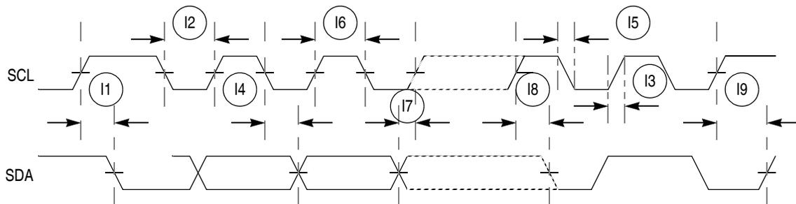
**Figure 8. I<sup>2</sup>C Input/Output Timings**
